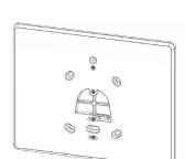
2. Attach the RE667 Slimline Touchpad wall mount at the locations shown below using the included hardware. Cover the holes indicated by applying the included overlay.
