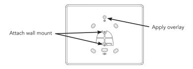
3. Attach the RE663 LED Keypad wall mount at the locations shown below using the included hardware.
