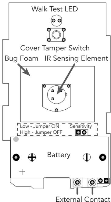
**Motion lockout** is active for three minutes after a motion event is detected. Motion events will be ignored during the motion lockout period.
