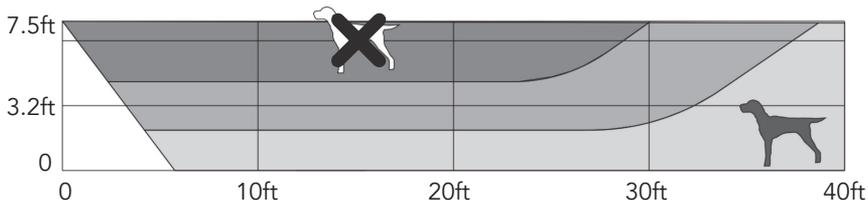
**Motion catch performance** is best when the motion sensor is positioned so a person would typically walk across the front of the motion sensor instead of directly toward the motion sensor.
