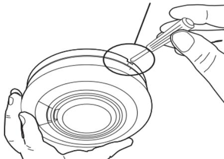
If necessary it is possible to further secure the Alarm by using a No.2 or No.4 (2 to 3mm) (1/8") diameter - not supplied) self tapping screw 6 to 8mm (1/4") long (see Figure 7d), to firmly lock the Alarm and its mounting plate together (see Figure 7c).
