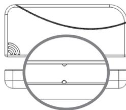
**Install** by removing the adhesive paper and adhering the NanoMax and magnet on a door or window. Make sure to align the alignment marks on the NanoMax and magnet when mounting. Alternatively, NanoMax can be used with an external contact instead of using the reed switch.
