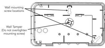
(Mounting hardware not included. Use two #4 or # 6 screws for mounting)
