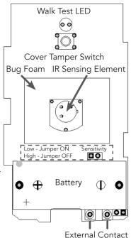
**Motion lockout** is active for 30 seconds after a motion event is detected. During the motion lockout period, motion events will be ignored.
