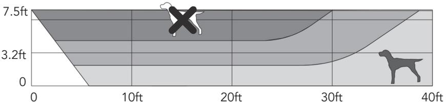
**Motion catch performance** is best when the motion sensor is positioned so a person would typically walk across the front of the motion sensor instead of directly toward the motion sensor.
