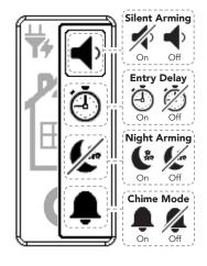
**Change Keypad settings** using the extended menu. Hold **MENU until** the Keypad chirps three times (roughly 3 seconds) to open the extended menu.
