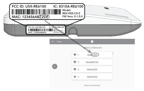
By default the Touchpad network list will show Connect+ and BAT-Connect access points. To view all networks in range tap the "Show all networks" button at the bottom of the network list.
