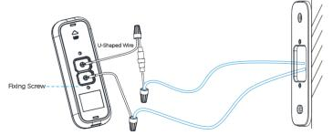
7 Fix the doorbell to the mounting plate by inserting the doorbell screws.
