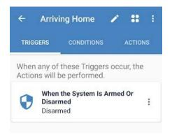
This scene will unlock the front door and turn on the living room lights (action) when the system is disarmed (trigger) when it is between sunset and sunrise (condition).
